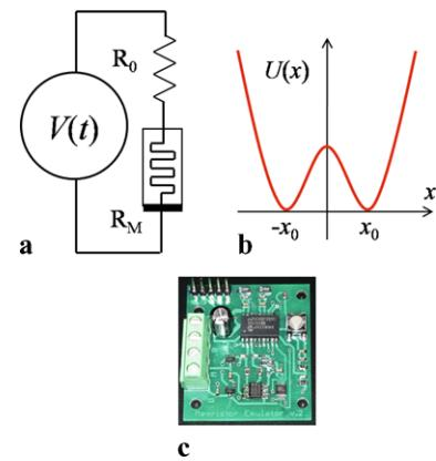
**Fig. 1** (a) Electronic circuit used in chaos measurements consisting of the programmable voltage source  $V(t)$ , 510 Ohms resistor  $R_0$  and memristor  $M$ . The memristor specifications are given in the text. (b) Schematic of the double-well potential governing the memristor. (c) Optical photograph of memristor emulator
