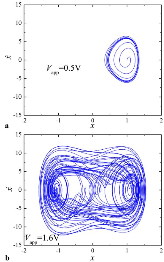
**Fig. 5** System trajectories below (a) and above (b) the chaos onset. These plots represent 50 s of system evolution driven by an applied ac voltage of 2 Hz frequency. The voltage amplitude is shown on the plots for each case
