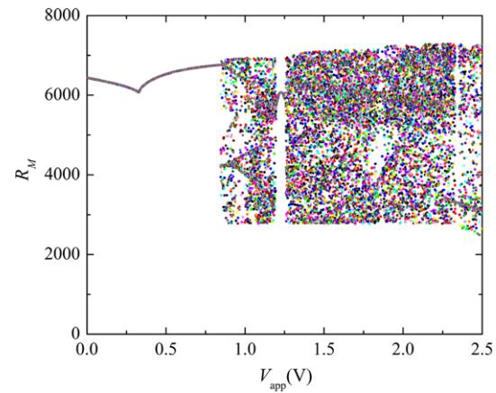
**Fig. 4** Numerically calculated value of memristance  $R_M(t_f)$  at  $t_f = 19.875$  s. This is plotted as a function of the amplitude of the applied voltage  $V_{app}$ . The fact that small changes in  $V_{app}$  (i.e., neighboring x-axis points) result in large changes in  $R_M(t_f)$  is an indicator of chaos
