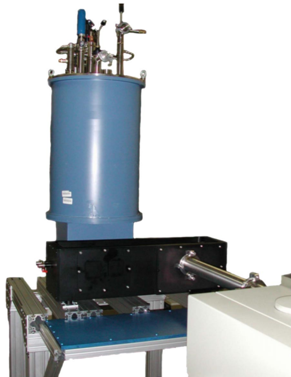
FIG. 2. (Color online) Photograph of the 9 Tesla superconducting magnet connected to the Michelson interferometer. The units are connected by 750cm of evacuated guide. The platform is where the detector would sit for reflection experiments. A similar box sits on the opposite side of the magnet for transmission (not shown).
