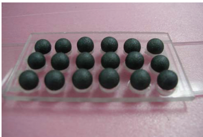
Fig. 5 MM constructed from natural materials, magnetodielectric spherical particles embedded in a matrix, which exhibits an NI.
