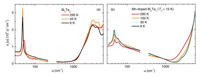
FIG. 4. (Color online) Infrared conductivity spectra  $\sigma_1(\omega)$  of Bi<sub>2</sub>Te<sub>3</sub> (a) and the Mn-doped Bi<sub>2</sub>Te<sub>3</sub> sample (b) at select temperatures. The data are cut near 300 cm<sup>-1</sup> due to a phonon in the GaAs substrate that eliminates transmission over this frequency range.
