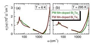
FIG. 6. (Color online) Infrared conductivity spectra  $\sigma_1(\omega)$  of the FM Mn-doped Bi<sub>2</sub>Te<sub>3</sub> film and a PM Mn-doped Bi<sub>2</sub>Te<sub>3</sub> film at 6 K (a) and room temperature (b).
