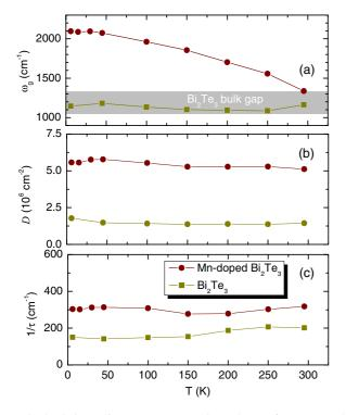
FIG. 5. (Color online) Temperature dependence of  $\omega_g$  (a), Drude oscillator strength *D* (b), and free carrier scattering rate  $1/\tau$  (c). The gray region in panel (a) covers the frequency (energy) range of values reported in the literature for the bulk band gap of Bi<sub>2</sub>Te<sub>3</sub>.
