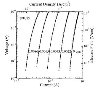
Fig. 5. E-J characteristics (circles) of a  $YBa_2Cu_3O_7$  microbridge measured at a fixed reduced temperature of  $0.79T_C$  after successive doses of ion damage. The solid lines are fits to the data using (4). The quality of the fits suggest that quantum fluctuations are responsible for the onset of dissipation.
