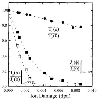
Fig. 1. The variation of  $T_c$  and  $J_c$  with ion damage in YBa<sub>2</sub>Cu<sub>3</sub>O<sub>7</sub> thin films.  $J_c$  is much more sensitive than  $T_c$  to ion damage. That  $T_c$  decreases with ion damage indirectly lowers  $J_c$  measured at a fixed temperature such as 77 K. The dashed lines are guides to the eye.
