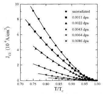
Fig. 6. The critical current density,  $J_{C2}$ , obtained from fitting E-J characteristics at several levels of ion damage and over a range of temperature. The solid lines indicate that  $J_{C2} \propto (1-T/T_C)^{3/2}$  at all levels of ion damage.
