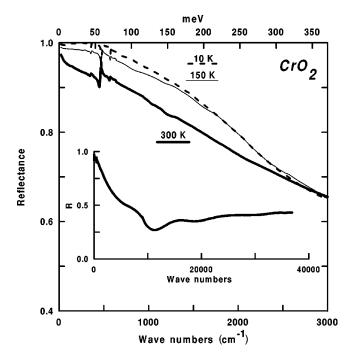
FIG. 1. Reflectance of  $CrO_2$  at 10 K, 150 K, and 300 K. Far-infrared reflectance is strongly temperature dependent and increases by as much as 7% at  $500 \text{ cm}^{-1}$ . The inset shows the 300 K reflectance over a broader energy scale.
